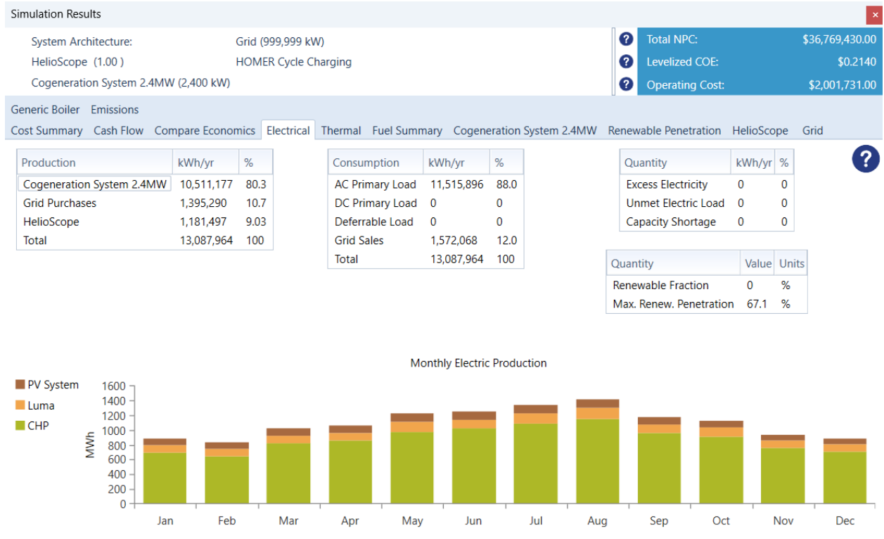
Figure 15.23: Homer Simulation Results LUMA, PV System and CHP (After Cogeneration Plant with PV System).
