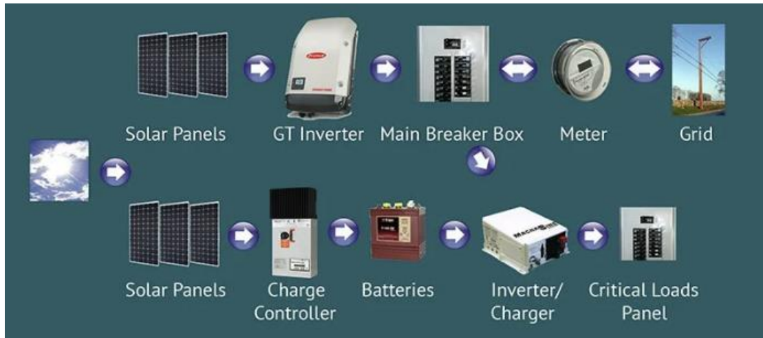
Figure 3.3: PV System Components
